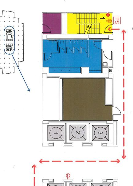
07/04/12 ©2008 AK Productions LLC (S) 7. Exit Stairwell with Designation Elevator Car with Designation Exit Route A ⊕ PS Freight Elevator with Designation **Pull Station** Standpipe Outlet Firemen's Phone Outlet Electrical Closet Restroom Mechanical Room Telephone Closet
