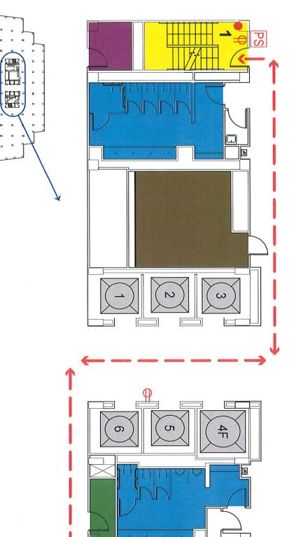
07/04/12 ©2008 AK Productions LLC (M) 72 HALL Elevator Car with Designation Exit Stairwell with Designation Exit Route A ⊕ PS Freight Elevator with Designation **Pull Station** Standpipe Outlet Firemen's Phone Outlet **Electrical Closet** Telephone Closet Restroom Mechanical Room
